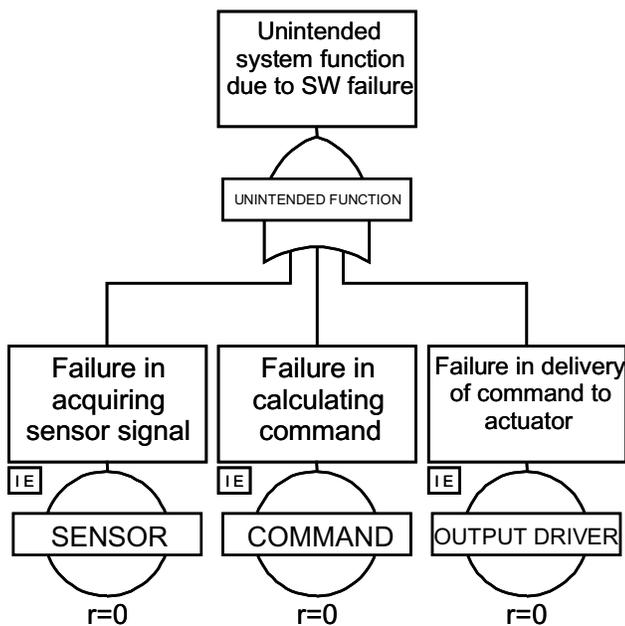
**Figure 3: System-Level Fault Tree for the Example Control System.**
