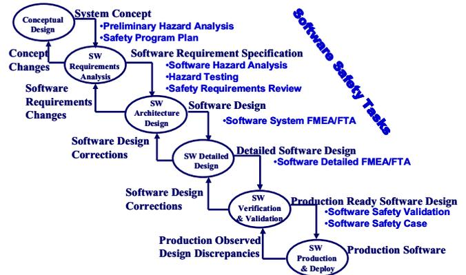
**Figure 1: Software Life Cycle with Associated Software Safety Tasks.**
