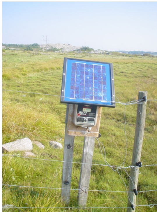
If there is no electricity available, a solar cell and 12 V battery can power the fence.
